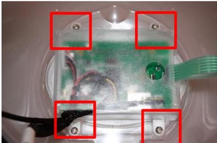
A photograph of a micro card with a clear plastic cover. Four red boxes highlight the screws that hold the cover in place. <ul style="list-style-type: none"><li>○ Débranchez les 2 connecteurs du câble de connexion.</li></ul> |  | Tournevis |
