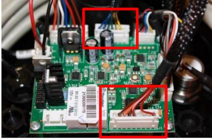
A photograph of a green PCB with various components. Two red boxes highlight the datalink cable connectors on the board.                                                                                                                                    |  |           |
